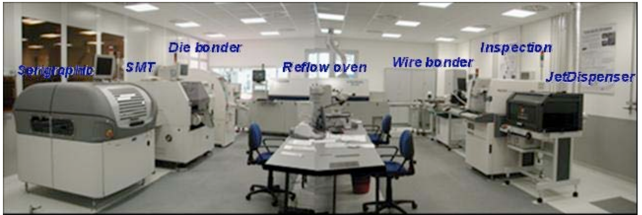
Figure 10. COB automatic assembling line at CRP labs.
