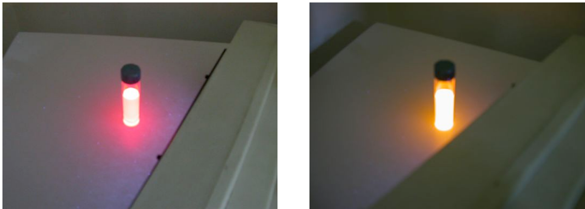
Figure 9. Red and yellow emitting particles in solution under standard UV lamp irradiation
